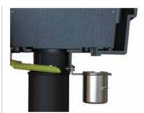
Mount the grease cup holder to the rear flange hold with a 1/4-20 x 3/4" bolt and 1/4-20 Kep nut. The grease cup holder is supplied with the grill head.
